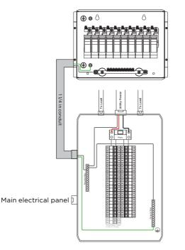
2. Connect L1 phase and L2 phase of the main electrical panel to corresponding inputs of SHP. Output wires of SHP are connected to corresponding hot wire terminals.
