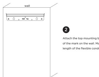
Attach the top mounting bracket along the top edge of the mark on the wall. Make sure you also check the length of the flexible conduit.
