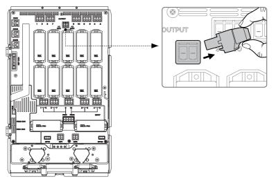
2. Connect L1 phase and L2 phase of the main electrical panel to corresponding outputs and inputs of SHP (L1 phase to 1, 3, 5, 7, 9 of SHP; L2 phase to 2, 4, 6, 8, 10 of SHP).
