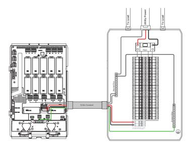
2. Connect input wires from SHP to corresponding breakers of the main electrical panel and output wires to the load port of the main electrical panel.
