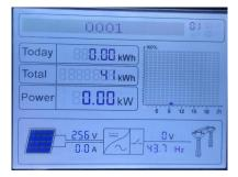
Press "OK" to enable Reflux Power, then input the Reflux Power value, press "Up" or "Down" to change the number, press "OK" to go to next digit.after this, press "OK", "success" is displayed when the Reflux Power is correct.
