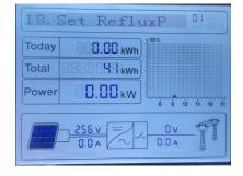
Select "Set RefluxP", press "OK", then "Input Password" will be displayed, press "OK" again to input the password (0001), press "Up" or "Down" to change the number, press "OK" to go to next digit.
