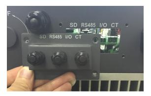
Step 3: Insert the other end of Network cable through the cable gland and waterproof.
