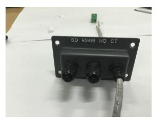
Step 4: Connect Network cable and CT port, secure the wires using a slotted screwdriver.
