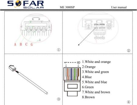
The logic interface pin definitions and circuit connections are as follows: Logic interface pin are defined according to different standard requirements
