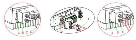
Step 1:Loosen 4 screws(A)using a screwdriver(Fig.4-2);
