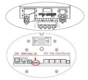
**Step 2** Press the SD card and take it out.Insert the SD card into a micro-SD card reader,then insert micro-SD card reader into a PC;(NOTE:micro-SD card reader&PC are not provided by SOFARSOLAR).
