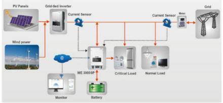
Fig.1-1 ME 3000SP schematic diagram
