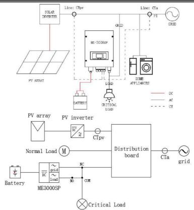
**Step 1**:Location of CTa:L wire of incoming mains.Location of CTpv:L wire of PV inverter' s output.
