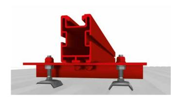
The K2 Bridge is mounted on two solar fasteners instead of the adapter plate in order to achieve greater span widths. Depending on type, the rail is fixed to the Bridge with one or two M10x30 T-bolts.
