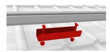
Lay Mounting Rail on joint with rail connector and connect with T bolts and self-locking nuts. The rail joint may not be in the range of the roof fastener.
