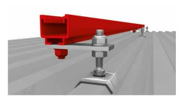
Ensure correct position of T-bolt. After inserting into the lower chamber of the rail, the T-bolt is turned 90 degrees counterclockwise. Lock the projected K2 module carrier rail Solid on the adapter plate with an M10 T-bolt and tighten. Tightening torque: 32 Nm
