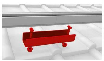
Lay Mounting Rail on joint with rail connector and connect with T bolts and self-locking nuts. The rail joint may not be in the range of the roof fastener.
