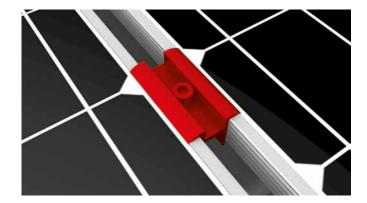
Use two universal module middle clamp OneMid between two modules. Klick the Stance in the notches. Place clamps on the module frames and fix them. Tightening torque 14Nm.
