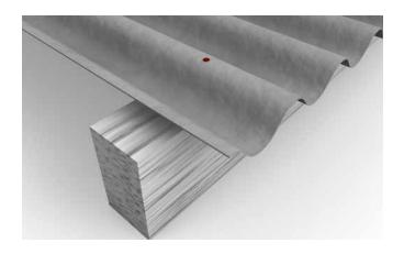
Measure the screw distances according to statics or K2 Base. Check position of purlins and pre-drill through the fibre cement profiles into the purlins.
