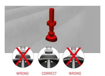
**Additional information:** Do not tighten the solar fastener with the torque, the seal must be slightly compressed and rest on the entire surface.
