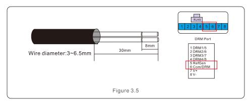
When the RJ45 terminal is connected with Solis logic interface, the 5th and 6th cable of RJ45 terminal should be connected with external control unit.
