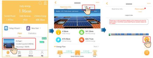
Log in to https://intl.fusionsolar.huawei.com to access the WebUI of the FusionSolar Smart PV Management System. On the Homepage page, click the plant name to go to the plant page. Select Plant layout. Choose ⊕ > Generate with AI, and create a physical layout as prompted. You can also manually create a physical location layout.
