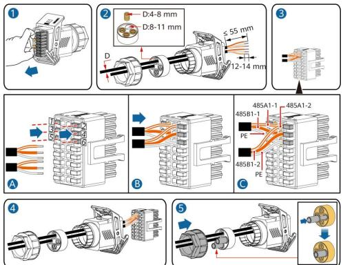
2. Connect the signal cable connector to the communication port.
