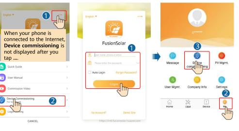
2. Connect to the solar inverter WLAN and log in as **installer** to access the device commissioning screen.
