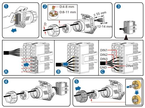
2. Connect the signal cable connector to the Communication port.
