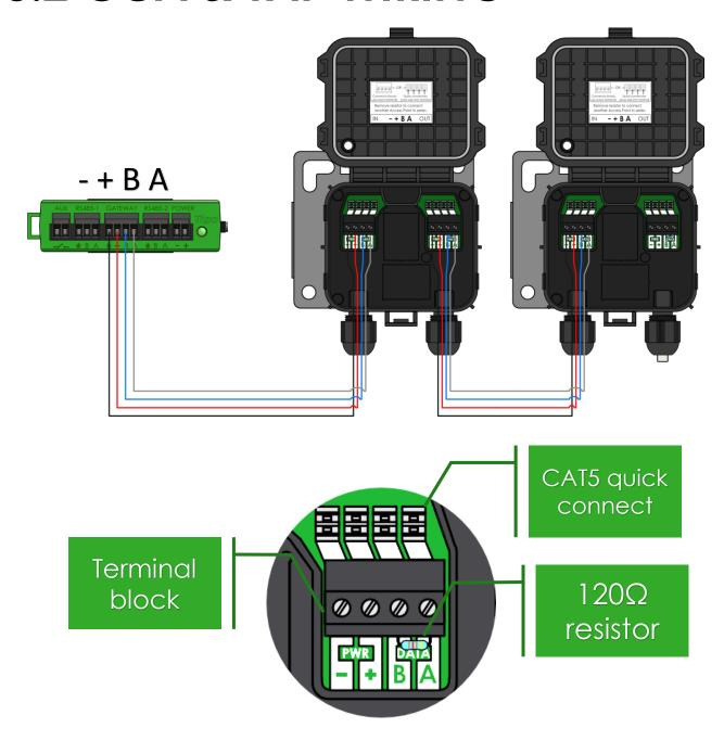
Connect multiple TAP units in series and leave terminating resistor only in final TAP.
