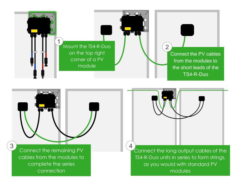
Note: connect modules to TS4-R-Duo inputs before connecting outputs
