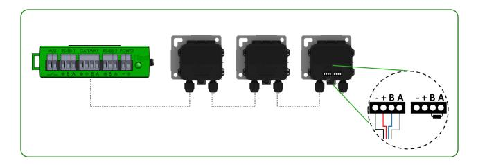
Connect multiple TAP units in series and leave terminating resistor only in final TAP only.
