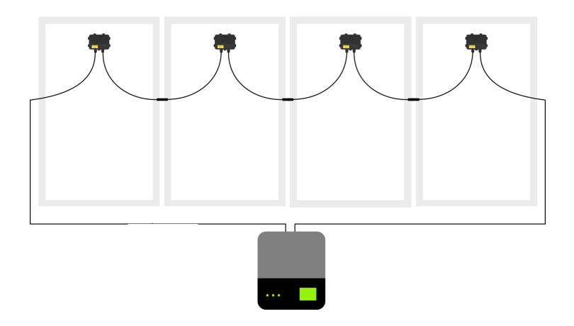
Smart Modules with Integrated TS4 Junction box are installed just like standard PV-Modules.
