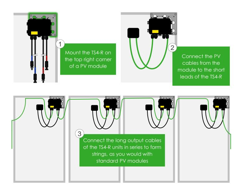
Note: connect modules to TS4-R inputs before connecting outputs
