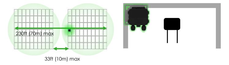
Place TAP within 10m of any TS4 unit in the array, with a maximum distance of 10m between TS4 units and 35m from TAP to farthest TS4.
