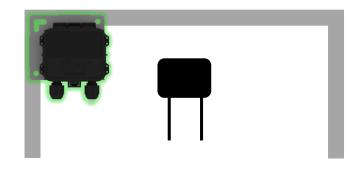
Place TAP near center of array or each sub-array
