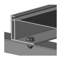
Figure 1. PV module installed with Bolt fitting method
