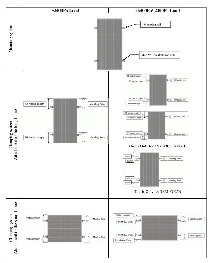
Other mounting configurations can be used. However, failure to comply with the above recommendations will result in a lowering of the load handling (snow/wind load) capabilities below the product specification 5400/2400Pa(IEC), 5400/3800Pa(UL1703) and product failure as a result of an overload situation will not be covered by the Trina Solar warranty.
