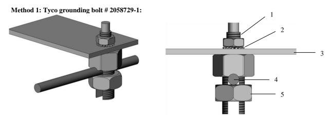
Figure 4. Tyco grounding bolt # 2058729-1
