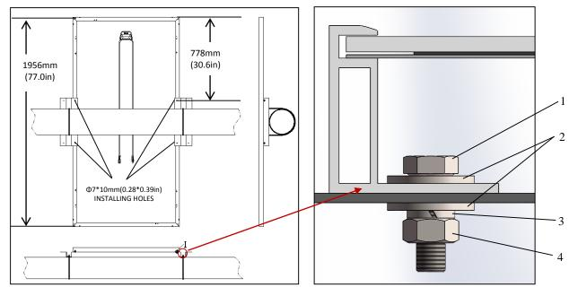
Figure 3. PV module installed with Single-axis Tracing System
