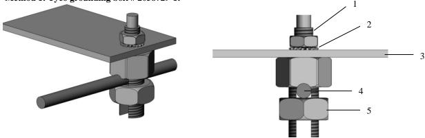
Figure 4. Tyco grounding bolt # 2058729-1
