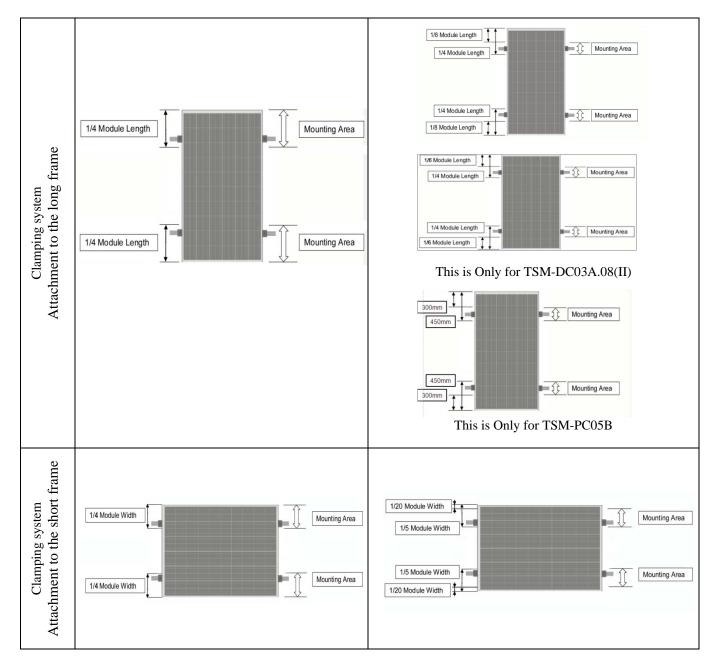
Other mounting configurations can be used. However, failure to comply with the above recommendations will result in a lowering of the load handling (snow/wind load) capabilities below the product specification 5400/2400Pa(IEC), 5400/3800Pa(UL1703) and product failure as a result of an overload situation will not be covered by the Trina Solar warranty.
