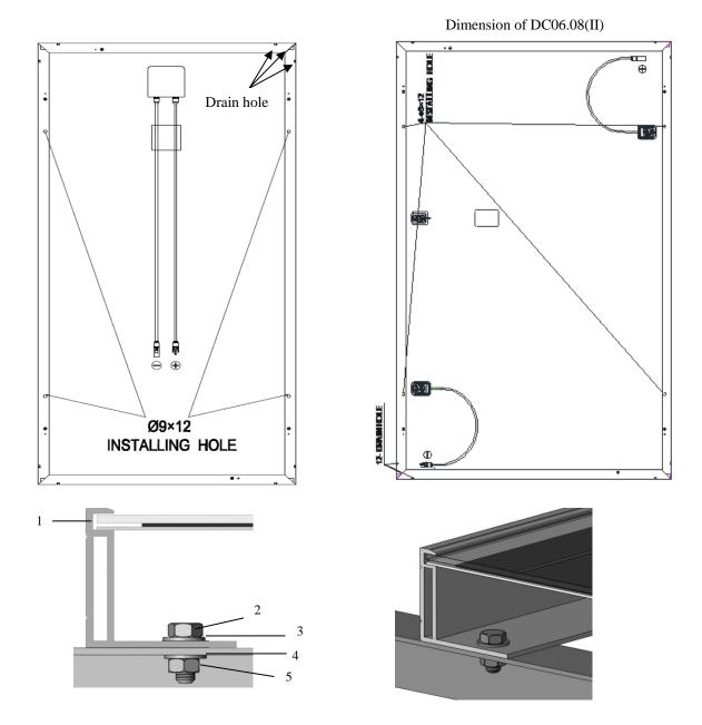
Figure 1. PV module installed with Bolt fitting method
