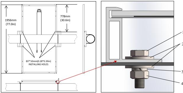
Figure 3. PV module installed with Single-axis Tracing System
