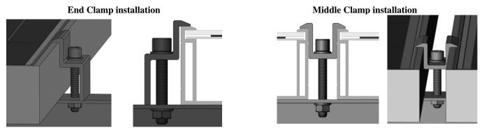
Figure 2. PV module installed with clamp fitting method
