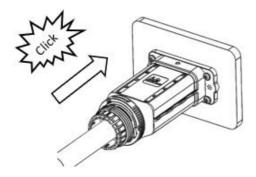
5. Tighten the nut with an open-ended wrench and complete the installation with a "click, click, click", then complete the installation.
