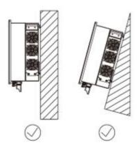
12. Never install the inverter horizontally, or with a forward tilt or with a backward tilt or even with upside down. The horizontal installation can result in damage to the inverter.
