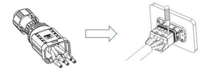
4. Insert the main body into the rubber core and hear the "click" sound.
