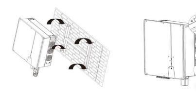
4. Secure the inverter to the mounting bracket on both sides using two M5 screws. Screwdriver type:PH2, torque:2.5Nm.
