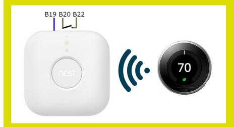
Then set the heat pump to use it as the signal to heat or not by setting **FSV 2091** - External Thermostat Application #1 (Floor) to
