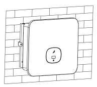
After confirming the inverter is fixed reliably, fasten one M4 safety-lock screws on the right or left side firmly to prevent the inverter from being lifted off the bracket.
