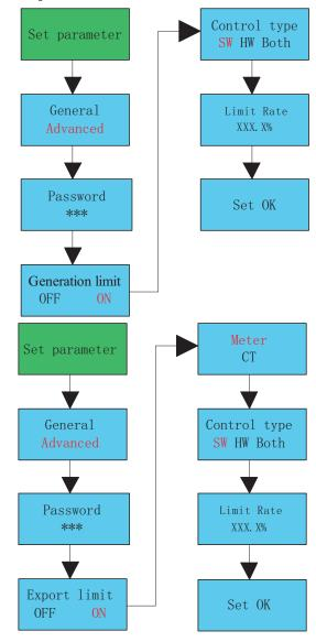
Under the permission given by your energy provider, the ratio of your system output power divided by the rated power of the inverter is called Limit Rate.For instance, if the energy provider only accepts 8kVA/kW from your 10kW system, then the Limit Rate of 10kW inverter is 80.0%.
