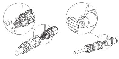
**Step 2** Push the threaded sleeve into the socket, Tighten up the cap on the terminal.
