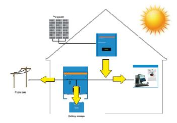
In this situation the grid is present and connected to the loads. The inverter/charger will see that the PV system is producing more energy than needed by the loads, resulting in a surplus of solar power. The surplus is used to charge the battery. All energy that is not absorbed by the battery, because it is fully charged or already being charged with the maximum charge current, is fed back into the grid.
