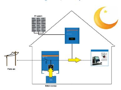
After a couple of days of monitoring PV power, the inverter/charger will synchronize its internal clock to the day/night rhythm. The inverter/charger will, without interrupting the AC supply, disconnect from the grid during the night and all energy for the AC loads will be drawn from the battery.
