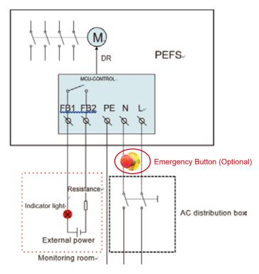
Resistor is selected according to supply voltage, to ensure circuit current less than the rated current of the Indicator light and < 320 mA
