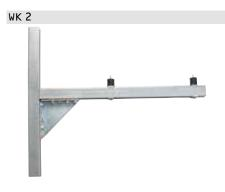
Corrosion-protected wall mounting support made from zinc-plated steel for on-site installation. Height adjustments can be made on the wall rail, while the appliance rail provides the possibility to align the appliance. Standard delivery includes: 2 pce, incl. anti-vibration mounts.
