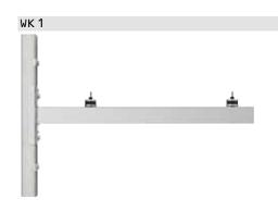
Corrosion-protected wall mounting support made from zinc-plated steel for on-site installation. Height adjustments can be made on the wall rail, while the appliance rail provides the possibility to align the appliance. Standard delivery includes: 2 pce, incl. anti-vibration mounts and 2 m ribbon heater.
