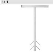
SK 1: Stainless steel, T-shaped support for floorstanding, concrete-embedded installation. Standard delivery includes: 2 pce incl. installation aid for a defined clearance dimension, anti-vibration mounts, plus 1 m ribbon heater. SK 2: White powder-coated bracket for installation on a strip foundation. Standard delivery includes: 2 pce incl. screws for securing the heat pump to the bracket.
