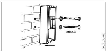
► Secure the lower insulation shell with the screws and washers supplied.
