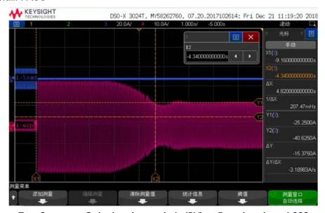
Test Category: Only the photovoltaic (PV) Reaction time: 4.82S
