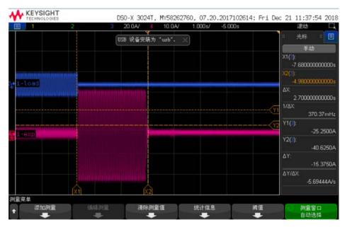
Test Category: Both batteries and photovoltaic cells Reaction time: 2.70S
