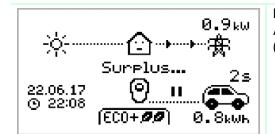
Enough surplus is available and zappi is about to charge the EV. A timer is decremented and can be set in the charge settings (ECO+ mode only).
